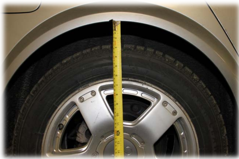
Figure 6: Measuring suspension heights prior to performing adaptation.
